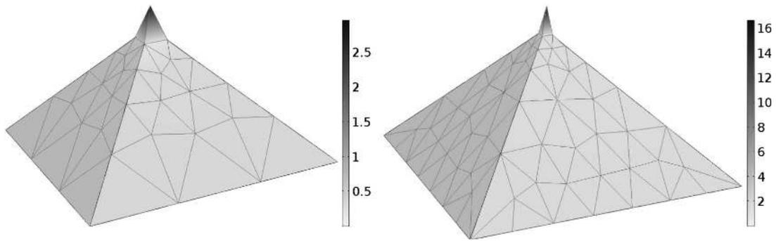
**Fig. 1.** Mesh-dependent solution for tip displacement with first-order elastic energy
