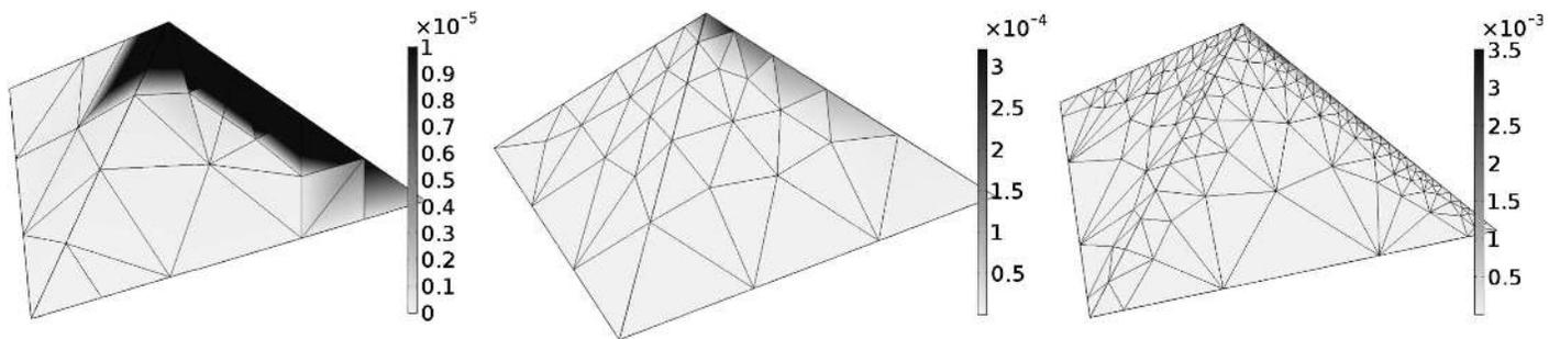
**Fig. 13.** Solution for a tetrahedron with prescribed nonconstant line displacement and fixed bottom surface equipped with the first-gradient energy (mapped in grayscale); the mesh becomes progressively finer around the edge with a prescribed line displacement
