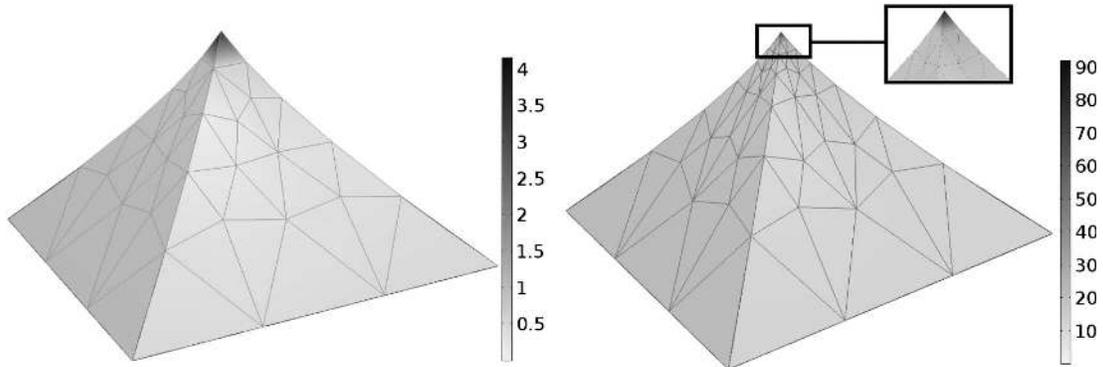
**Fig. 2.** Mesh-dependent solution for tip displacement with second-gradient elastic energy
