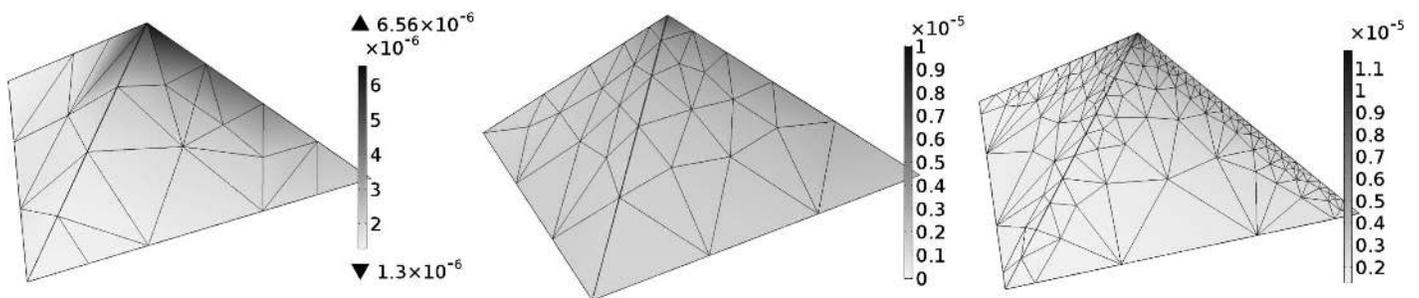
**Fig. 14.** Solution for a tetrahedron with prescribed nonconstant line displacement and fixed bottom surface equipped with the second-gradient energy (mapped in grayscale); the mesh becomes progressively finer around the edge with a prescribed line displacement
