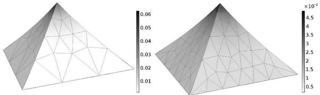
**Fig. 3.** Mesh-independent solution for tip displacement with third-gradient elastic energy
