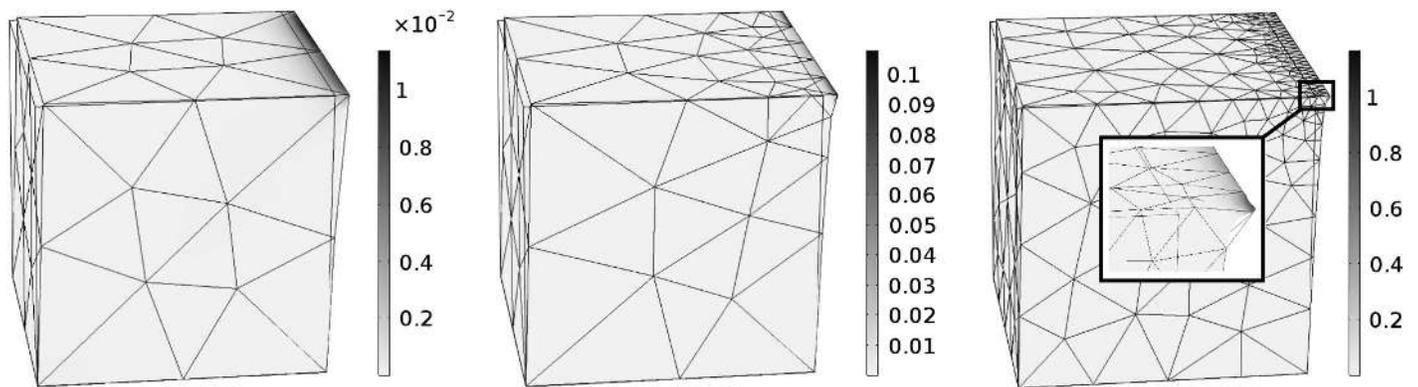
**Fig. 17.** Deformed cube with fixed bottom surface and prescribed displacement at one edge with the first-gradient energy; the mesh becomes progressively finer around the edge with a prescribed line displacement
