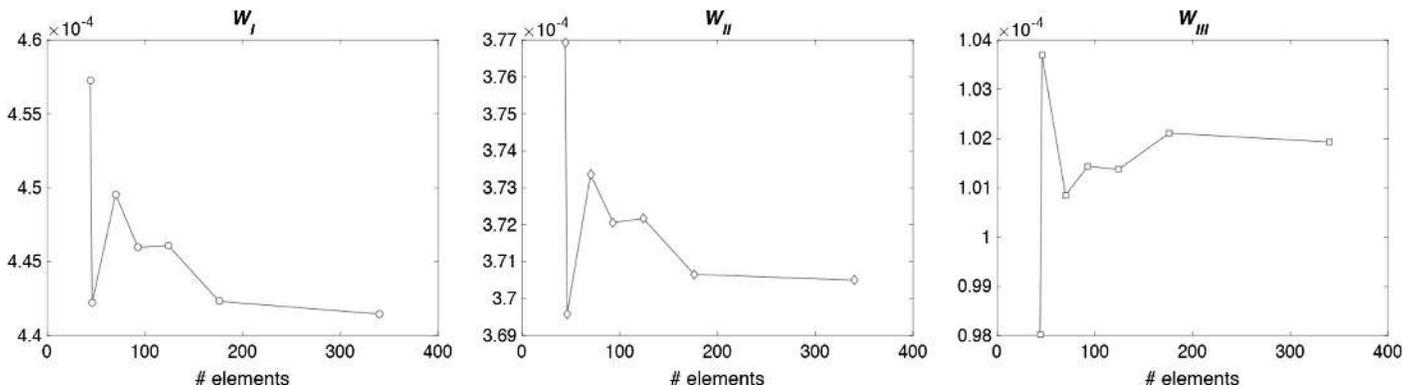
Fig. 6. Value of the components  $W_I$ ,  $W_{II}$ , and  $W_{III}$  of the stored elastic third-gradient energy  $W_{\text{grad}^3}$  for meshes with different number of elements
