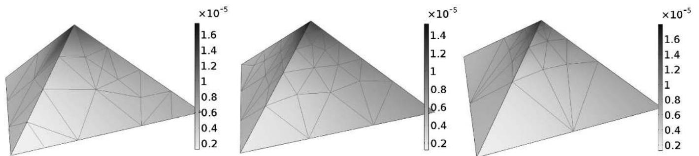
**Fig. 15.** Solution for a tetrahedron with prescribed nonconstant line displacement and fixed bottom surface equipped with the third-gradient energy (mapped in grayscale); the mesh becomes progressively finer around the edge with a prescribed line displacement
