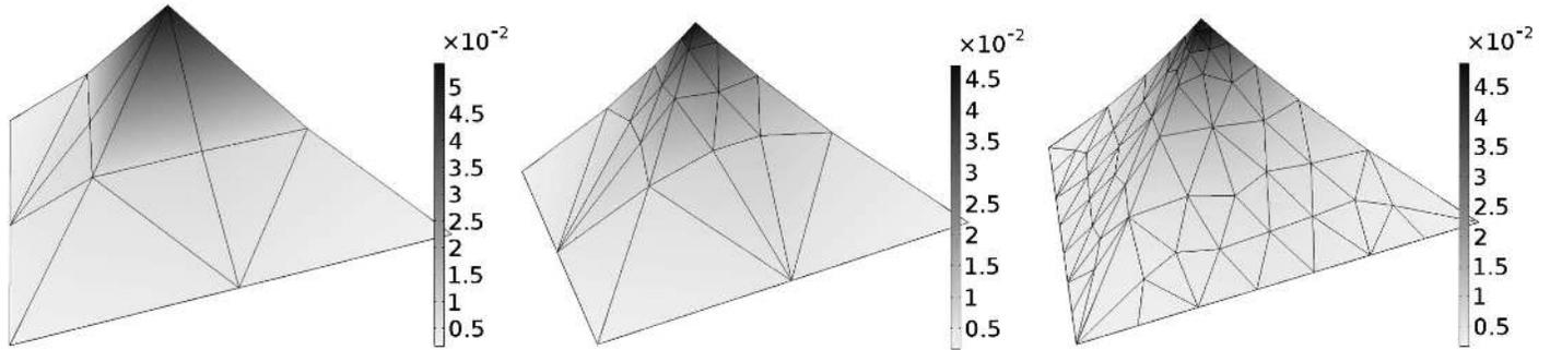
Fig. 5. Third-gradient energy: solutions for meshes with 46, 176, and 340 elements
