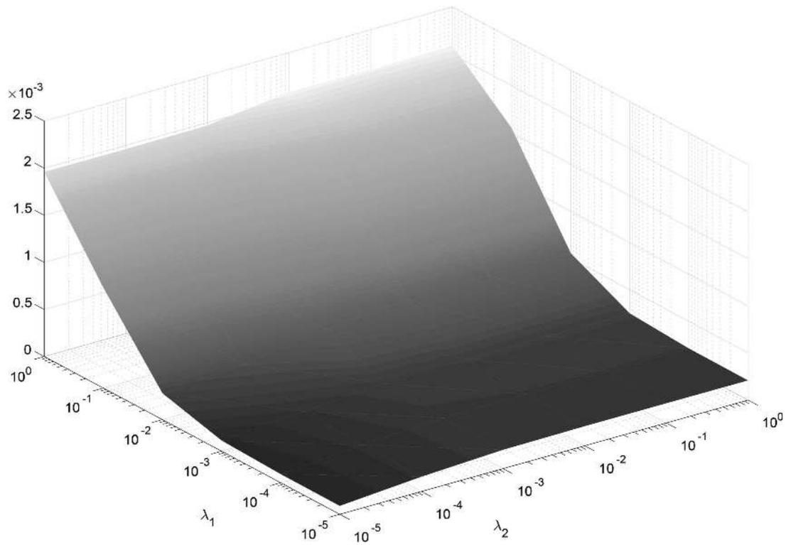
**Fig. 8.** Stored elastic third-gradient energy  $W_{\text{grad}^3}$  plotted over different ranges of  $\lambda_1$  and  $\lambda_2$
