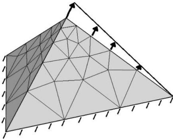
**Fig. 12.** Prescribed line displacement along an edge of a tetrahedron
