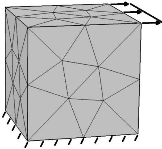
**Fig. 16.** Cube with fixed bottom surface and prescribed displacement at one edge
