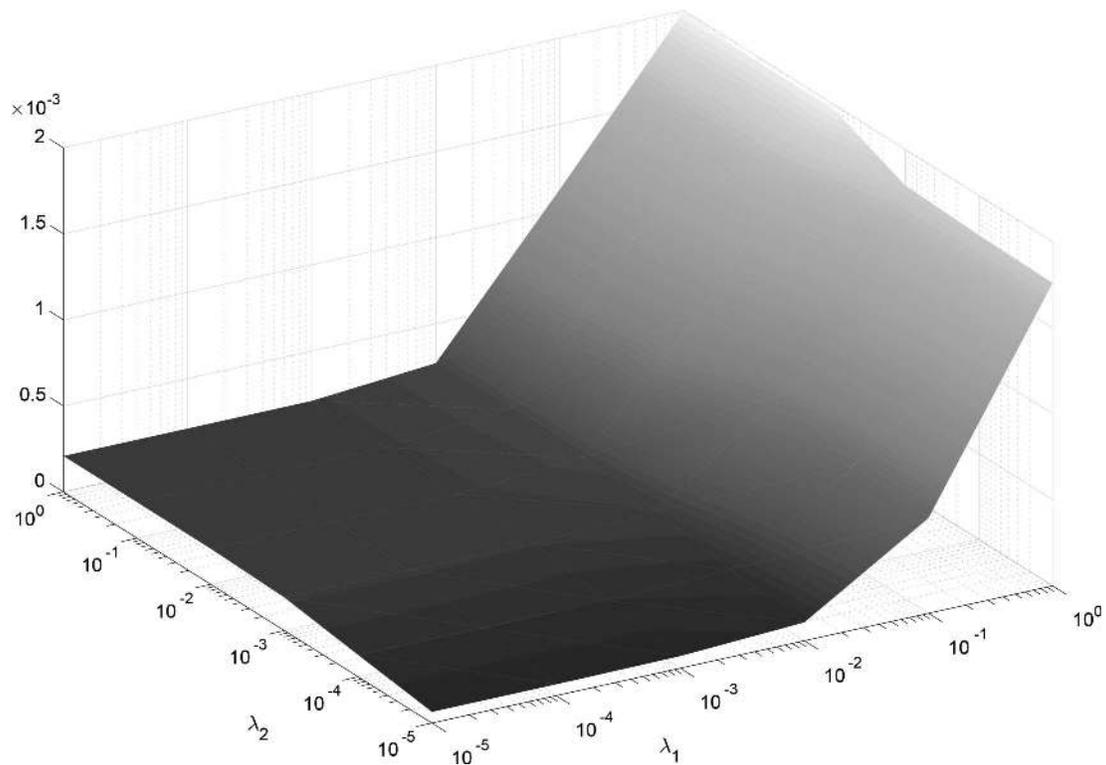
**Fig. 9.** Stored energy component  $W_I$  plotted over different ranges of  $\lambda_1$  and  $\lambda_2$
