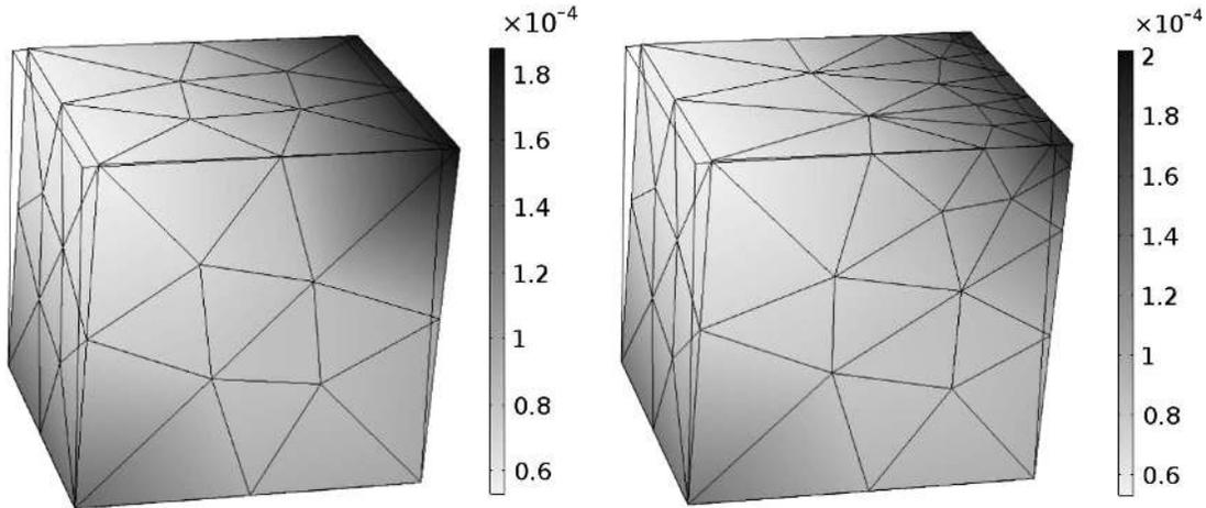
**Fig. 19.** Deformed cube with fixed bottom surface and prescribed displacement at one edge with the third-gradient energy; the mesh becomes progressively finer around the edge with a prescribed line displacement
