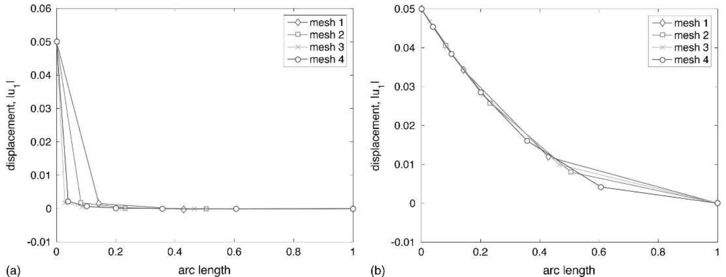
Fig. 7. Value of the amplitudes of the displacement component  $|u_1|$  in the case of (a) first-gradient energy; (b) third-gradient energy  $W_{\text{grad}^3}$ , for meshes with different number of elements
