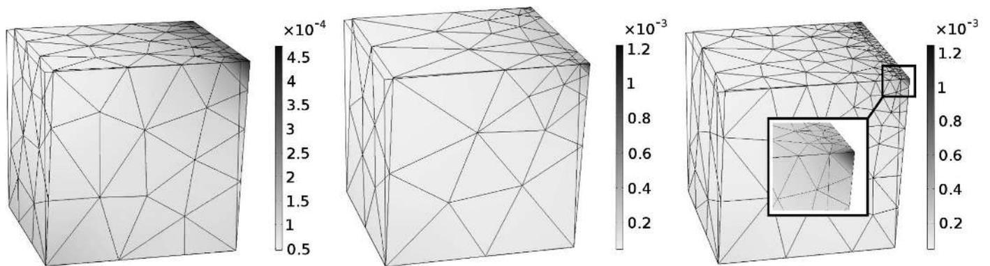
**Fig. 18.** Deformed cube with fixed bottom surface and prescribed displacement at one edge with the second-gradient energy; the mesh becomes progressively finer around the edge with a prescribed line displacement
