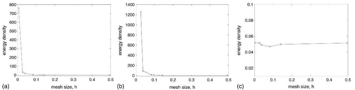
**Fig. 4.** Energy density versus mesh size at the tip of the tetrahedron for first-gradient, second-gradient, and third-gradient elastic energy models, respectively
